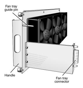
**3** Slide the fan tray into the chassis (Figure 5).
